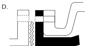
D. When installing a pinch valve to a rubber, PVC, or any "slick" mating flange, we recommend that you install a metal serrated gasket between the two flanges to assist in the seal.
