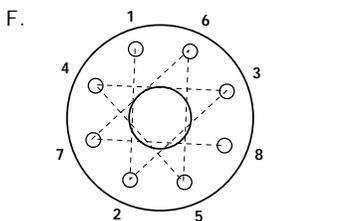
F. Torque all the flange bolts in a star pattern, first to 50% of tabulated valves, then retorquer to 100% of tabulated valves. If greater torque is required, continue retorquing in increments of 50% of tabulated valves. Use of high quality anti-seize compound on all bolt threads is recommended.
