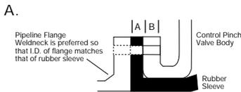
A. Standard pinch valves are built to schedule 40 pipe I.D. and to ANSI Class 125/150# flange and bolt circle specifications. It is recommended that the mating flanges are flat and full faced.
