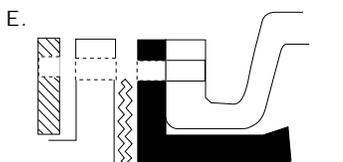
E. When bolting a pinch valve to a PVC or synthetic mating flange, use a split back-up retaining ring, since the mating flange will yield prior to generating enough force on the flange faces for a proper seal.
