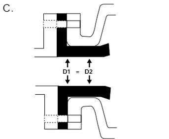
C. Mating flange ID must match the pinch valve sleeve ID.
