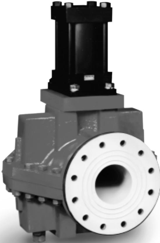
The Red Valve Series 9000 hydraulically actuated Pinch Valve is a bi-directional valve designed for tough slurry applications. The elastomer sleeve closes on entrapped solids in the line. The flexing action of the sleeve breaks up any sediment or build-up in the valve, which makes the Series 9000 a reliable, low maintenance valve.
