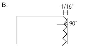
B. It is recommended that the mating flange be serrated to "grip" the rubber flange. The serrations should be cut 1/16" deep, with a 90 degree tool point. The pitch should be 8 (eight) cuts per inch.
