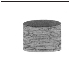
Figure 5. Wrong / Left: Rough striations indicate a dull cutter or too rapid feed. Correct / Right: Clean edges mean good cutting action.
